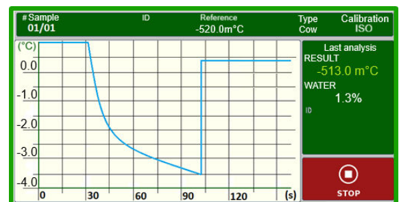
Real-time graph of the cryoscopic point measurement
